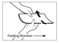
② If there is difficulty in straightening out curled paper, curl the front edges of the paper upward, as shown below.
